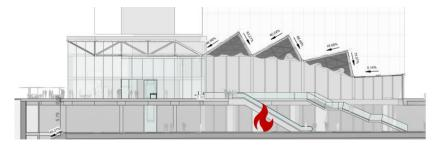
Figure 42. Diagram showing the smoke retention in the canopy gables.
