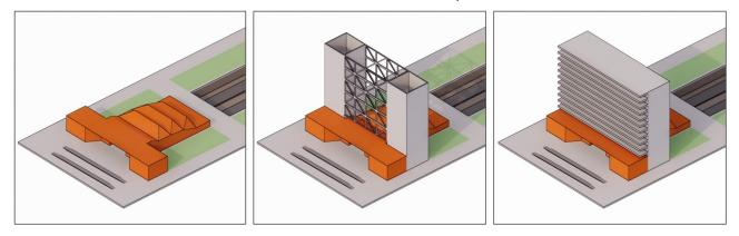
Figure 24. Schematic representation of the landmark building structure that will be needed to bridge the station entrance
