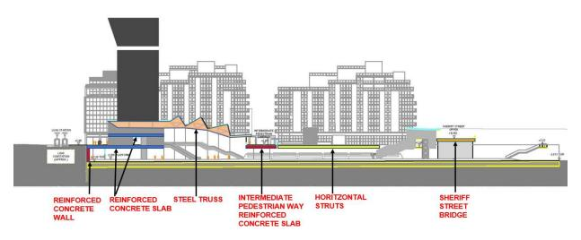
Figure 71. Longitudinal section. Structural systems
