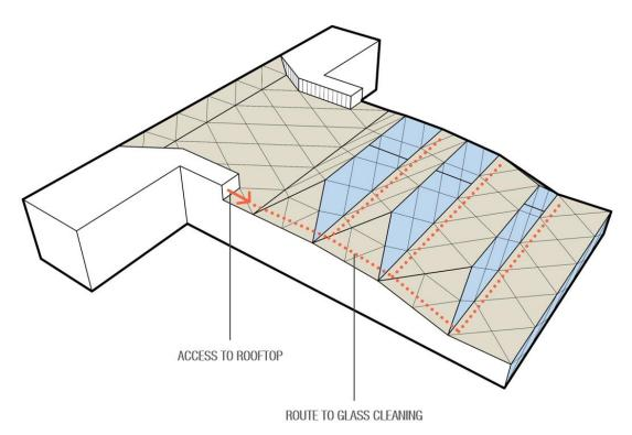
Figure 44. Diagram of the roof maintenance routes
