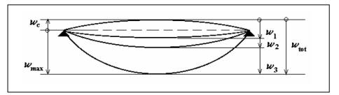
Figure 84. Definition of vertical deflections. (Source: I.S. EN-1990-2002+A1-2005, A.1.4.)
