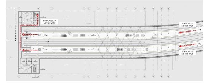
Figure 29. Platform level plan showing the emergency exit routes
