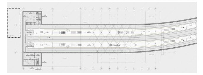
Figure 36. Functional layout of the proposed station at platform level
