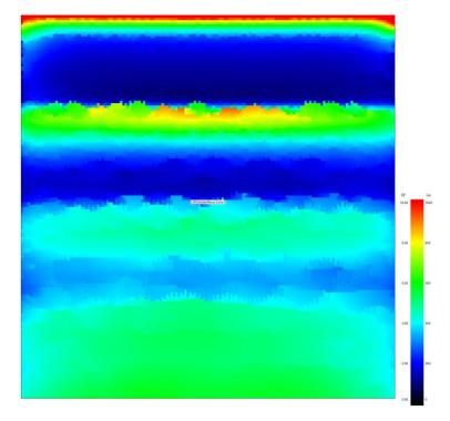
Figure 104. Station natural illumination study through the canopy skylights
