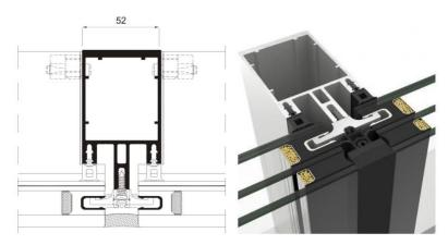
Figure 62. Section and photo detail of curtain wall.
