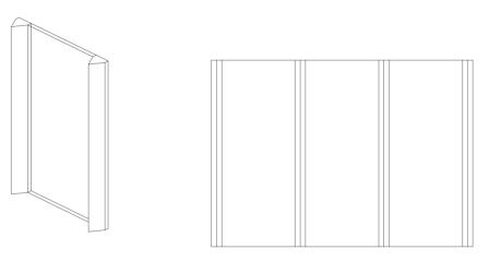
Figure 53. Axonometric and elevation view of vertical lamellas
