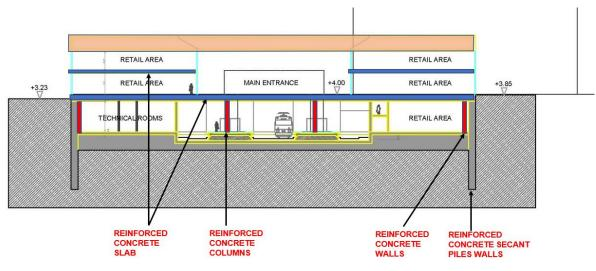
Figure 72. Cross section. Structural systems
