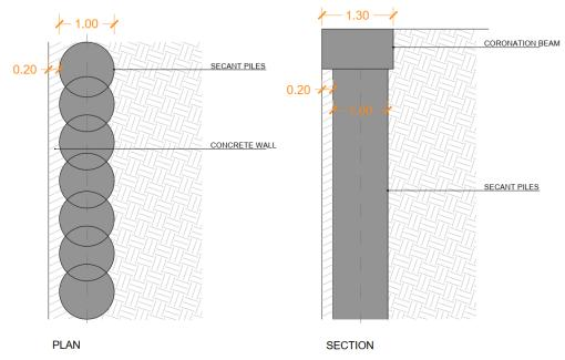
Figure 69. Sketch of secant piles
