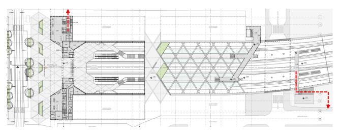
Figure 30. Street level plan showing the emergency exits to Park Lane and Abercorn Road.
