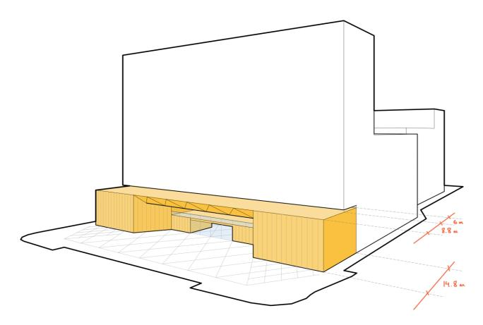
Figure 23. Dimensions of the alignment of the station with the alignment of the future landmark building.
