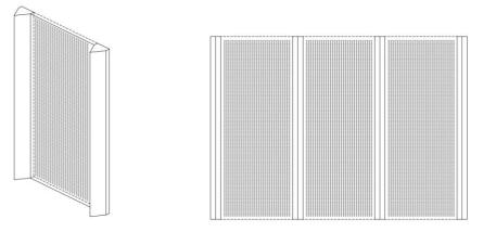
Figure 54. Axonometric and elevation view of vertical acoustic panels between lamellas
