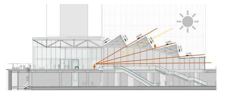
Figure 41. Diagram showing the gables adaptation to the passengers' views.
