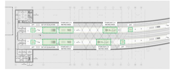
Figure 28. Platform level plan showing the vertical communication elements
