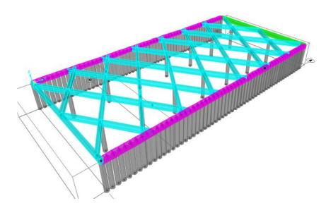
Figure 91. Structural numerical model of shoring system over Zone D
