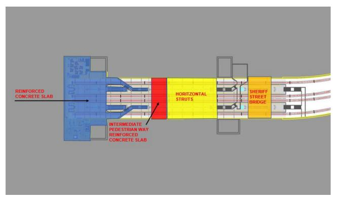
Figure 73. Platform Level. Slabs typologies
