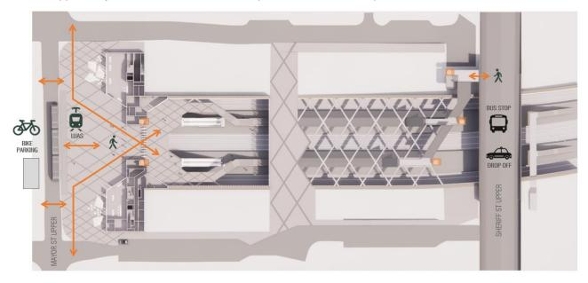
Figure 26. Diagram showing the intermodality and accesses to Spencer Dock Station
