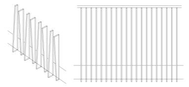
Figure 50. Axonometric and elevation view of the balustrade design
