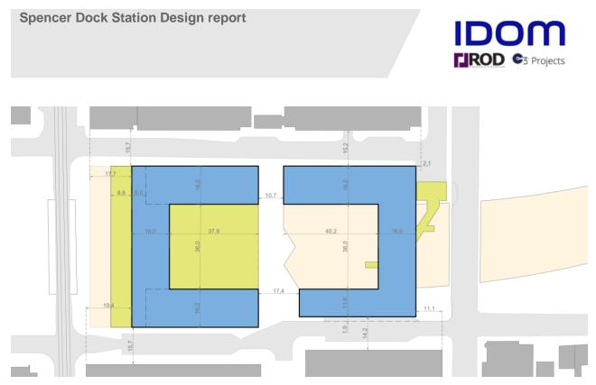
Figure 22. Dimensions and alignments of a possible configuration of the OSD (blue) integrated with the station design (green).
